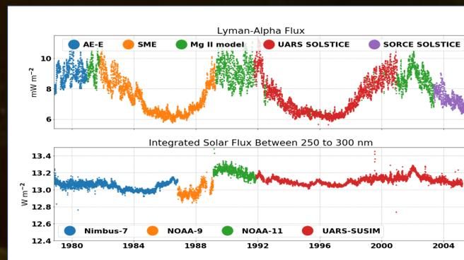
Solar Cycle Variations in the Lyman-Alpha (121.6 nm) and integrated 250 to 300 nm band. The difference in intensity at the shorter wavelengths is much more pronounced than in the 250 to 300 nm UV range.
