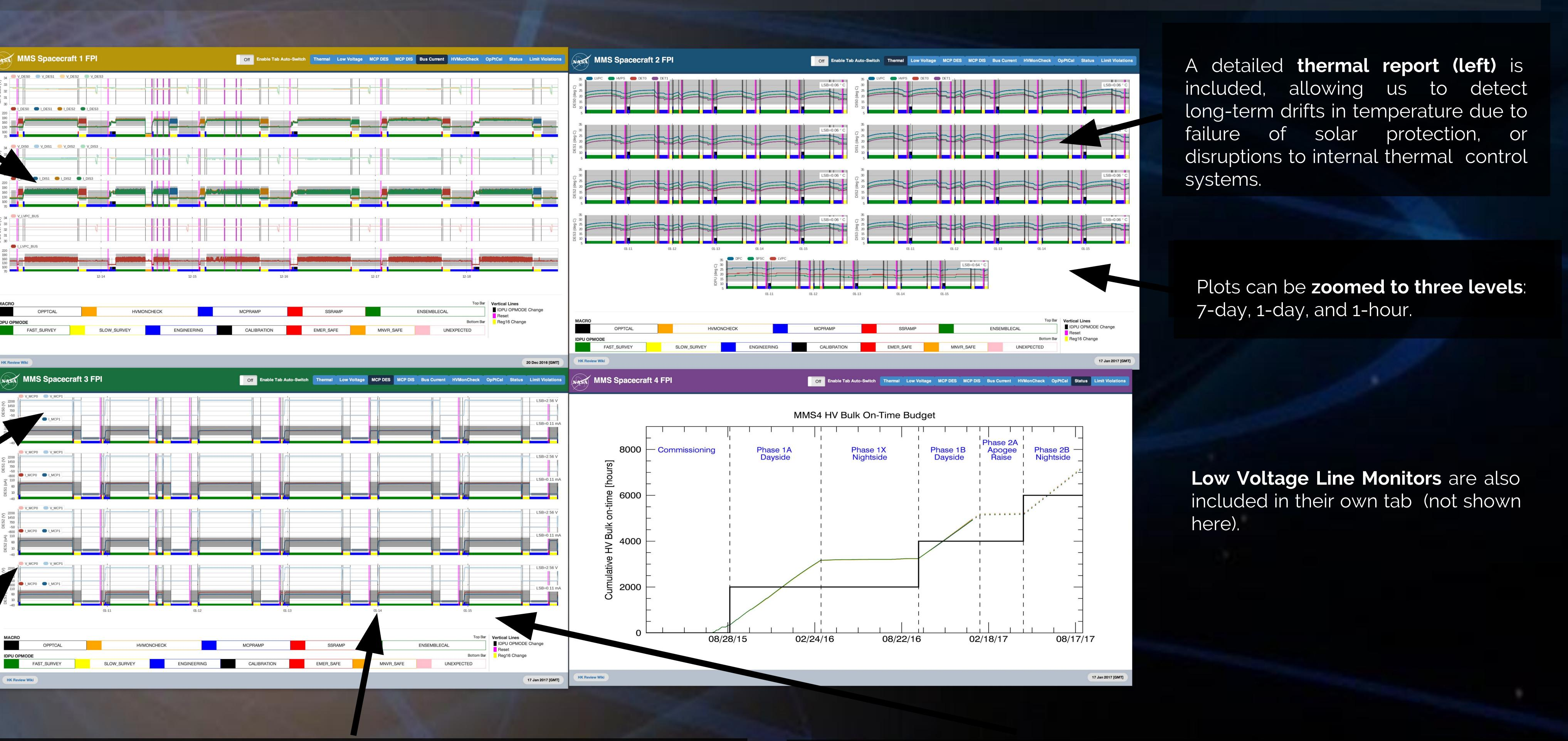
The dashboard is built using 100% open source technologies with no dependency on COTS software or languages requiring licensing fees. The overall framework is managed by Django, while the plotting and binary decoding are handled by Python. An in-memory cache is hosted by Redis. There has been discussion with the SpacePy developers around open sourcing the vectorized decoding algorithm for CCSDS packets and including it in the SpacePy library.
